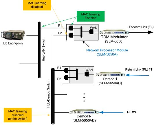
Figure 2: Bridged Point-to-Multipoint Block Diagram
